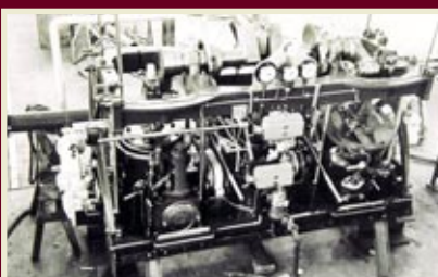
GISELA is the last boat operating an oscillating connected twin cylinder steam engine built in 1870.
